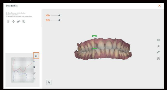
Various tools on the cross-section bar are designed to enhance your 3D view by allowing you to cut the model along the cross-section line you have drawn.
